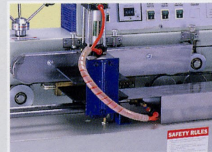
Hydraulic type: Provides a powerful compression effect. Recommended for expanded products, such as sponge ...etc.
